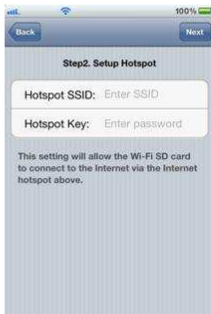
Step 2. Add an Internet Hotspot SSID and security key, then tap Next
