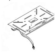
Thread open end of security strap (19) up through a slot on the outer edge of platform, across the platform, and then down through the other slot.
